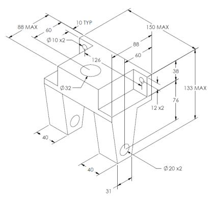
It is critical that all mounting holes and bearing holes remain in the same relative positions. The overall dimensions of the bezel cannot exceed 150mm x 133mm x 88mm. The 20mm and 32mm diameter holes are designed to accept standard bearings as shown:
