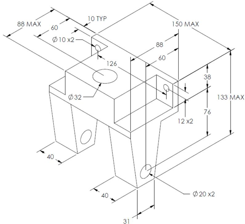
It is critical that all mounting holes and bearing holes remain in the same relative positions. The overall dimensions of the bezel cannot exceed 150mm x 133mm x 88mm. The 20mm and 32mm diameter holes are designed to accept standard bearings as shown:
